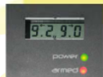
LCD ENERGISER OUT & RETURN VOLTAGE DISPLAY
